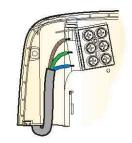
Firmly connect the conductors. Do not exert strain on the terminal block.
